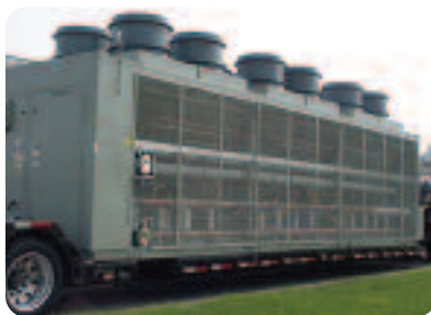
Air-cooled chiller with low noise condenser fan option to meet lot-line requirement of 68 dBA five feet from the unit.
